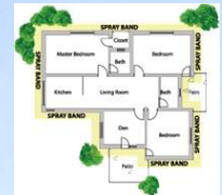
Perimeter pest control
